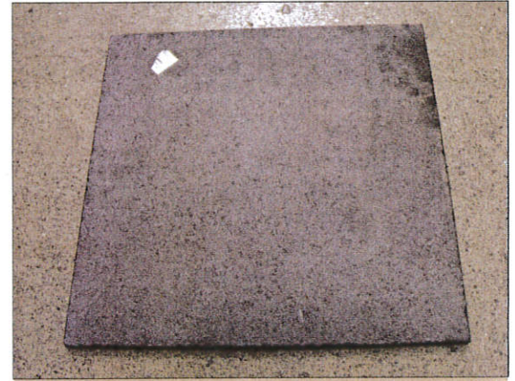
Black granite back side; rough surface profile in which light is diffused, resulting in low gloss and color.
